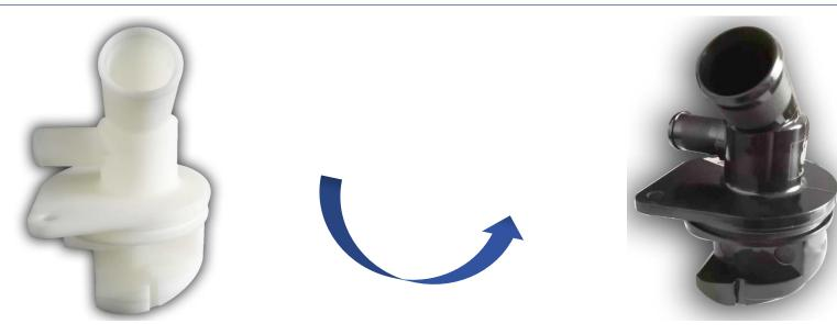
Nozzel Prototype by 3D printing
