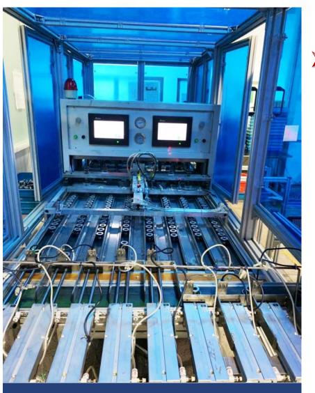
**Automatic Leakage Testing**
