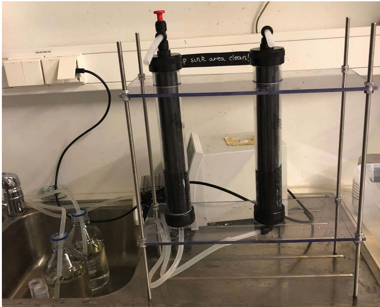
Figure 15: laboratory setup of Granular Activated Carbon filtration
