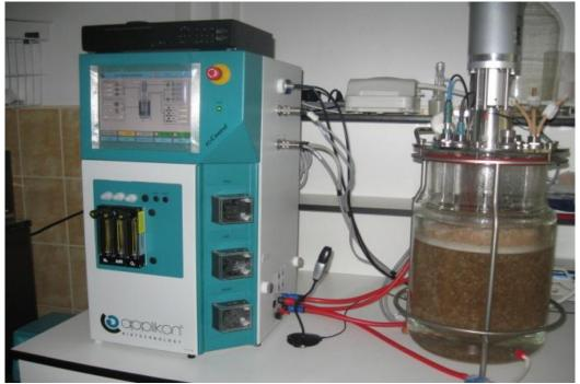
Figure 2: A setup of Submerged Fermentation for the production of secondary metabolites.
