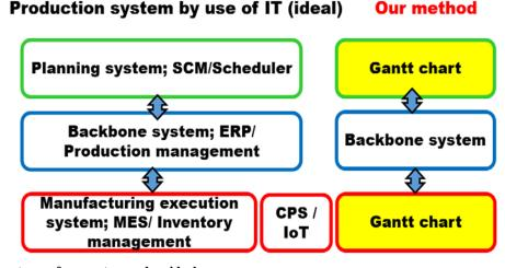
Fig. 4 System structures of our system and an ideal case.
