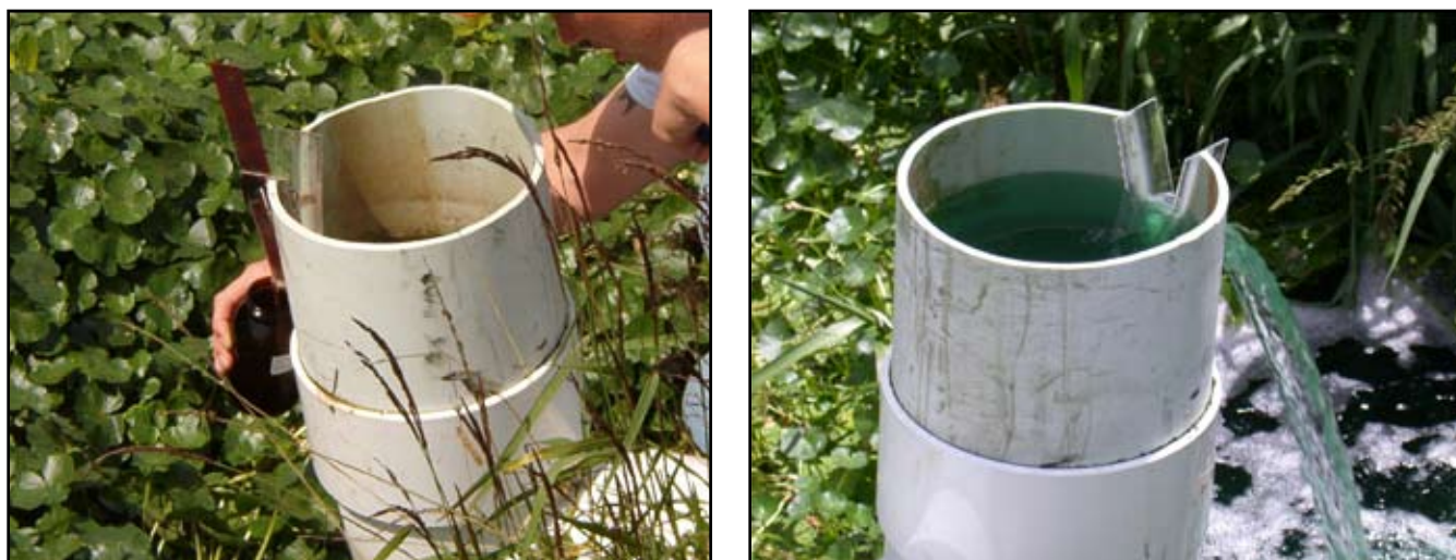
Figure 3. Water depth in notch estimates discharge rate from production area.
