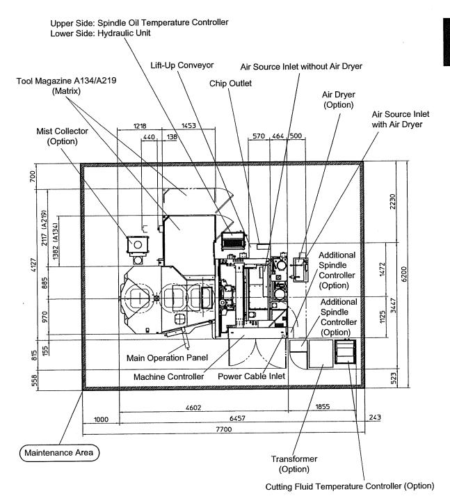
Figure 2.4 Top View of Machine (Tool Magazine A134/A219 and Left Discharge Type Lift-Up Conveyor Spec.)
