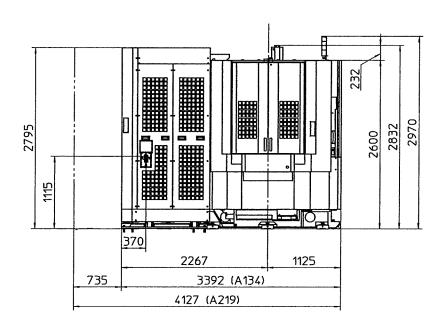
Figure 2.3 Front and Side View of Machine (Tool Magazine A134/A219 and Left Discharge Type Lift-Up Conveyor Spec.)
