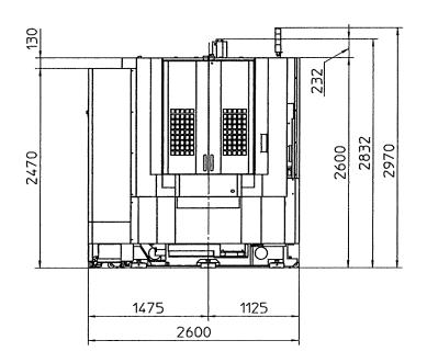
Figure 2.1 Front and Side View of Machine (Tool Magazine A40/A60 and Left Discharge Lift-Up Conveyor Spec.)
