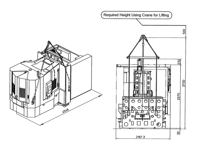
Figure 2.5 Main Machine When Being Transported
