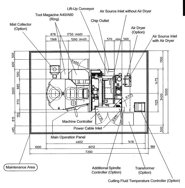
Figure 2.2 Top View of Machine (Tool Magazine A40/A60 and Left Discharge Lift-Up Conveyor Spec.)
