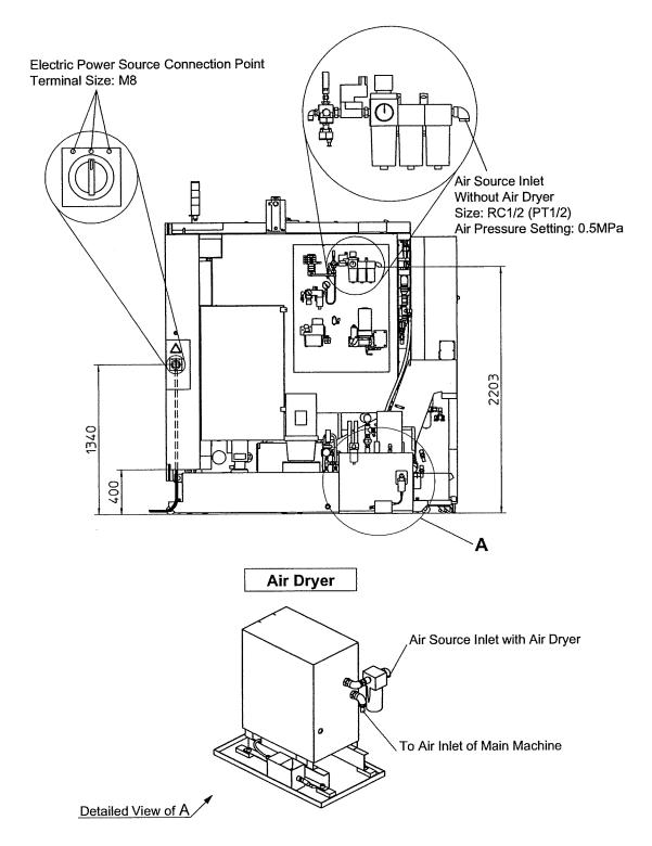
Figure 2.7 Power, Air Intake and Air Piping (with Air Dryer)
