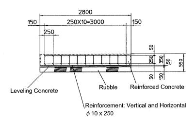
Figure 2.9 Foundation Drawing (Tool Magazine A134/A219 and Left Discharge Lift-Up Conveyor Spec.)
