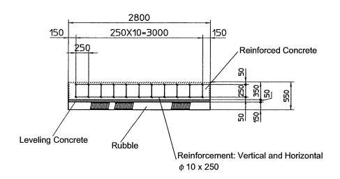
Figure 2.8 Foundation Drawing (Tool Magazine A40/A60 and Left Discharge Lift-Up Conveyor Spec.)
