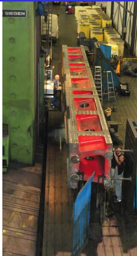
ALCOA: upper, cross and lower beams for one of the world's largest closed-die forging presses, 450 MN
