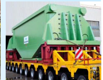
ALCOA: upper, cross and lower beams for one of the world's largest closed-die forging presses, 450 MN
