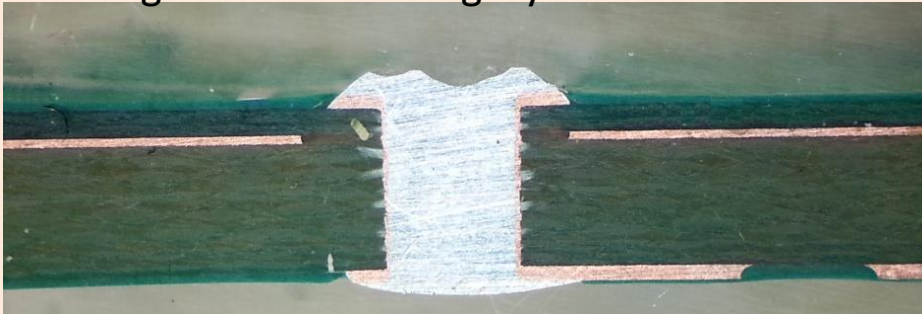
Image of PCB Showing layers and filled via
