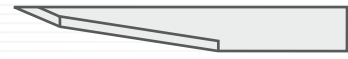
500-9810 - L25 Knife 65° - 80° Max cutting thickness (with gliding disc) - 5mm Max cutting thickness (without gliding disc) - 11mm
