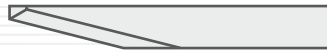
500-9813 - L25 Knife 0° - 65° Max cutting thickness (with gliding disc) - 5mm Max cutting thickness (without gliding disc) - 6mm
