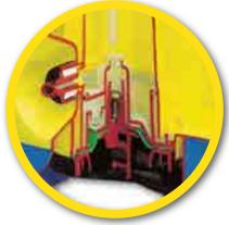
Thanks to its combined thickness and flexibility (specific technical plastic material: technopolymer), the CP diaphragm is highly hermetic and resistant, ensuring long-life and performance from the sprayer.
