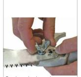
Replace lock washer and wing nut, tighten.
