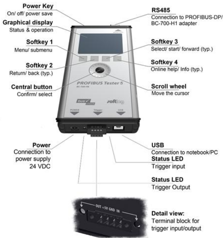
Figure 10: Connectors, buttons and status displays on the BC-700-PB
