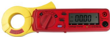
Figure 4: Fieldbus shield digital leakage current clamp
