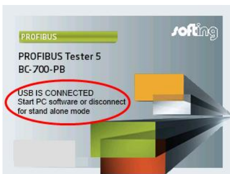
Figure 12: Power-up display when USB connected
