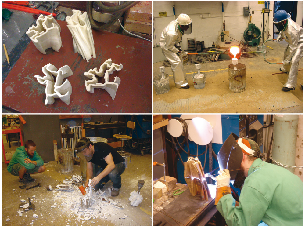
Fig. 8. Profilograph (after Muybridge). The digital model becomes 3D prints used directly in bronze investment casting. The bronze parts are welded together into a single form.
