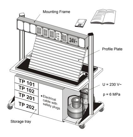
Fig. 1: Pneumatik 2000 – i.e. mobile workstation The modular design of the learning system permits applications beyond the limits of the individual packages. PLC actuation, for example, is therefore possible of pneumatic, hydraulic and electrical actuators.
