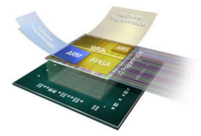
• Thanks to increased bandwidth between the processing system and the programmable logic, the new architecture delivers higher levels of programmable systems integration and performance at a fraction of the power consumption
