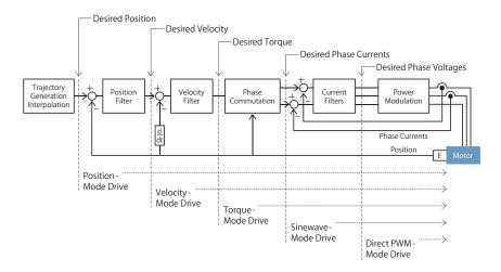
The PMAC has many modes for controlling motors: position-, velocity-, torque-, sinewave-, and direct PWM-mode drives. In addition to default servo algorithms, custom servo algorithms can be implemented. This enables motors to be fully synchronized even if many external devices are connected.
