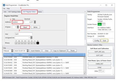
Figure 5.9. Read IO\_VDD\_SEL Bit from Device
