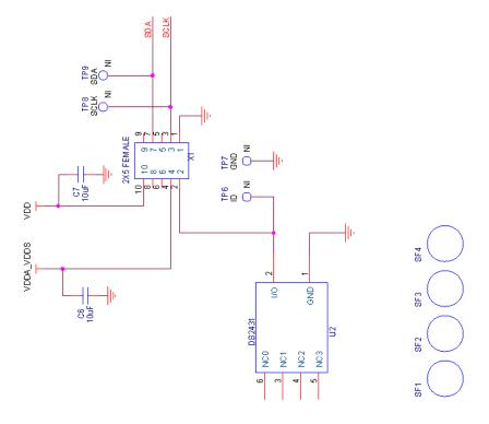
Figure 6.7. Si5332 48-Pin Socket Board Schematic
