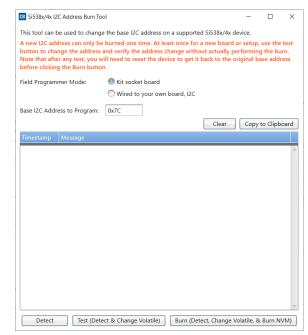
Figure 5.18. I2C Address Burn Tool
