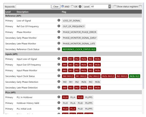
Figure 4.41. External Reference Valid but Inputs are Invalid and PLLs Not Locked
