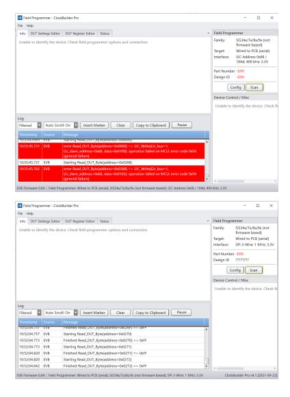
Figure 5.14. I2C and SPI Communication Failure Examples
