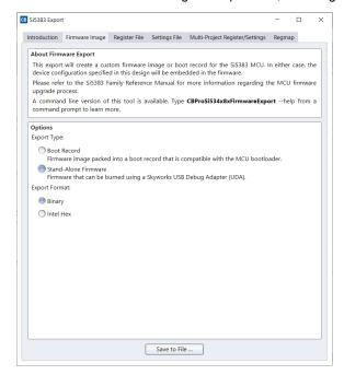
Figure 4.8. Stand-Alone Firmware Selection in the CBPro Export Menu for a Si5383 Device
