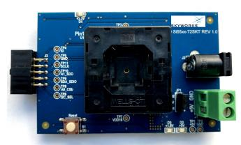
Figure 1.3. Si5332-32SKT-DK, Si5332-40SKT-DK, Si538x4x-44SKT-DK, Si5332-48SKT-DK, Si538x4x-56SKT-DK, Si538x4x-64SKT-DK, Si558x-72SKT-DK Sockets Sold Separately
