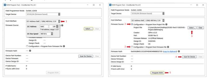
Figure 4.9. Programming In-socket, Firmware Based Devices
