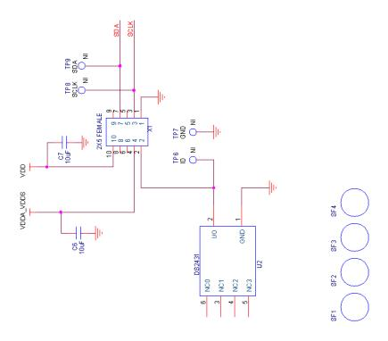
Figure 6.8. Si5332 40-Pin Socket Board Schematic
