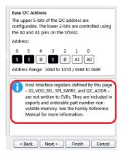
Figure 5.17. Base I2C Address
