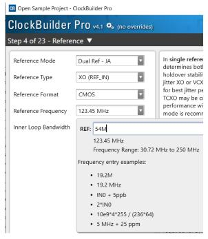
Figure 4.40. Correcting the Reference Frequency
