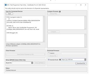
Figure 4.50. Select the Latest Field Programmer Firmware Image
