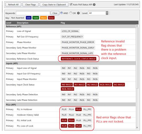
Figure 4.39. EVB GUI Reference Error Example, Si5518
