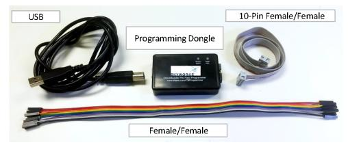
Figure 1.1. Field Programmer Kit Contents
