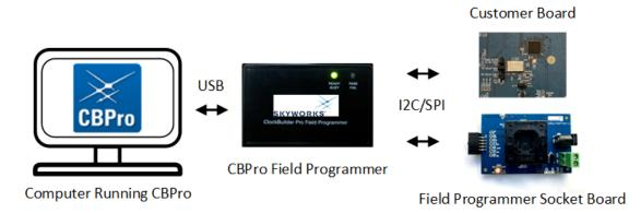
Figure 4.1. Computer to Field Programmer Connection
