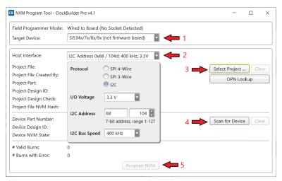
Figure 4.20. Programming In-system, Non-firmware Based Devices
