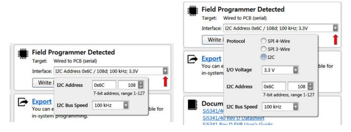
Figure 4.25. Communication Interface Selection
