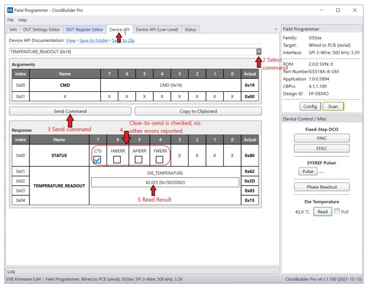
Figure 4.42. Si55xx API Command Example—Temperature Readout
