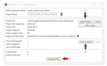
Figure 4.10. Programming In-socket, Non-Firmware Based Devices
