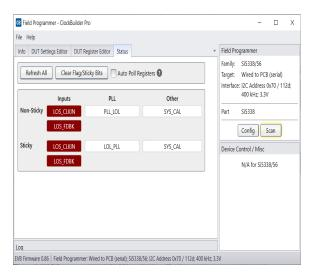
Figure 4.44. Reading Live Status Bits on the Si5332/8 and Si5350/1/7 Devices
