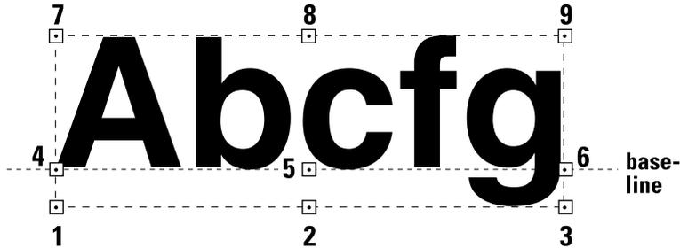
A text field makes up an imaginary box limited in regard of width by the length of the text, and in regard of height by the matrix size of the selected font. In text fields, the anchor points 4, 5, and 6 are situated on the base-line, as opposed to bar code fields and image fields.
