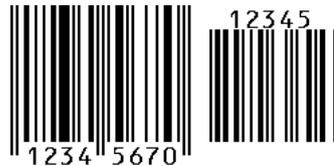
The AddOn code can be used in combination with any EAN and UPC bar code set. The following example prints a composite bar code, with a two-character AddOn code. More information on composite bar codes can be found later in this chapter.
