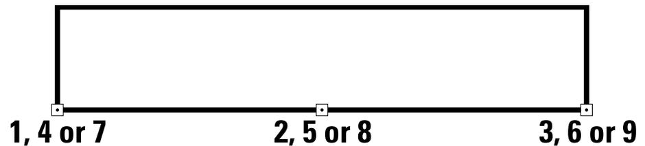
The anchor points are situated at the lower side of the line or box in relation to how text is printed in the selected direction. Lines and boxes have only three anchor points, each of which can be specified by means of three different numbers.
