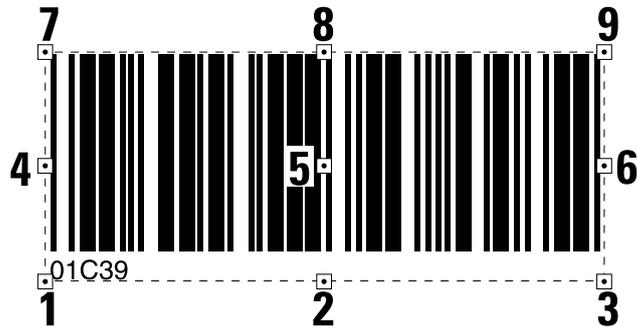
A bar code field makes up an imaginary box sufficiently large to accommodate the bar code interpretation, regardless if it will be printed or not (provided that the selected type of bar code may include an interpretation at all).
