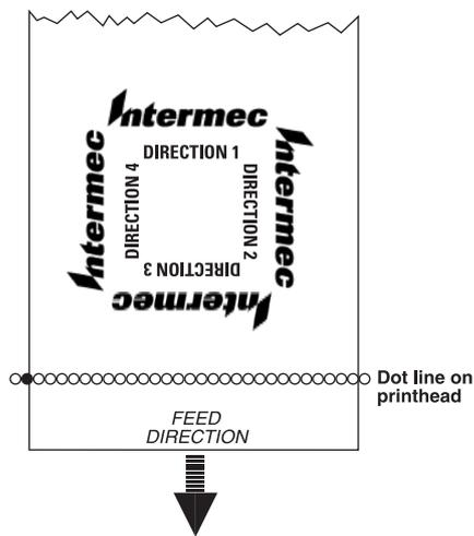
The relation of the image and the print direction depends how the image was drawn. An image can only be "rotated" 180°. Thus, it may be useful to have two copies of the image available with different extensions for either horizontal or vertical printing:
