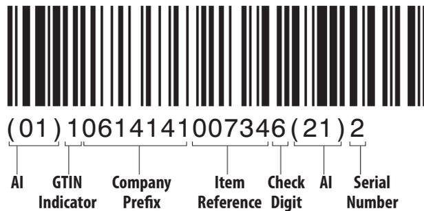
The Application Identifiers (AI) are dropped, as this information is included in the header. The check digit is dropped. The GTIN indicator is repositioned at the leftmost position of the item reference, to form a new item reference. A filter value of 3 is chosen for this example (signifying Standard Trade Item Group, though filter definitions are non-normative at this time). This gives us the necessary values to program an SGTIN-96 tag.
