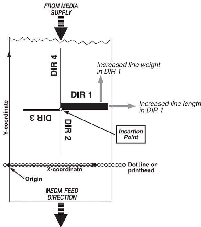
**Example** This example draws a 2.5 cm (1 inch) long and 10 dots thick line across the media in an 8 dots/mm printer:
