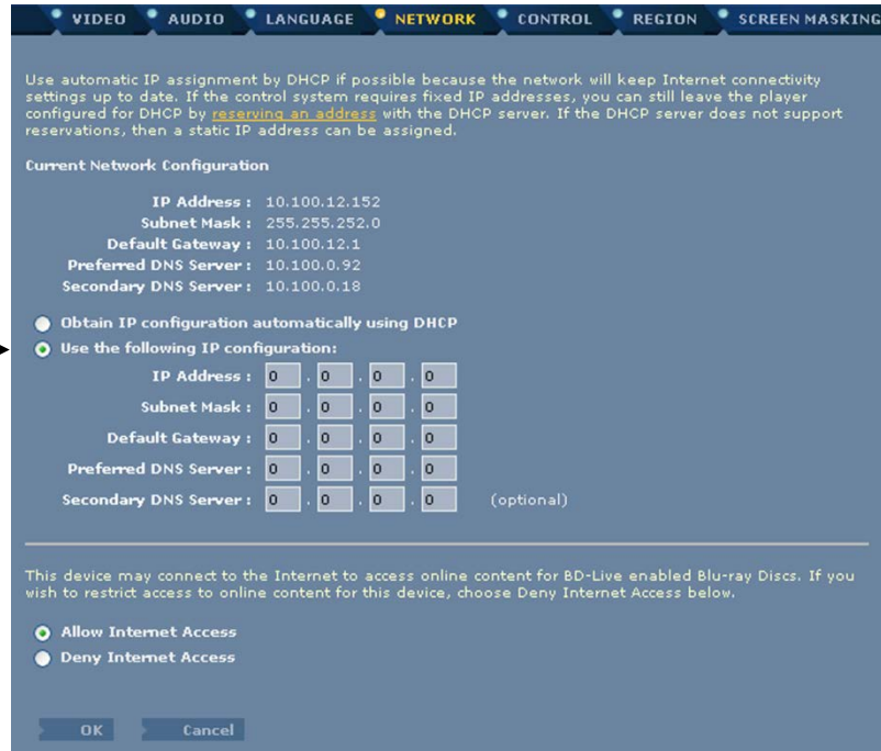
Figure 13: Static IP address assignment under the NETWORK tab
