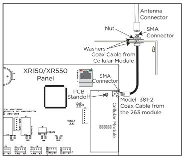
Figure 13: Cellular Module Installation
