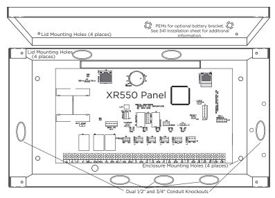
Figure 3: XR550 Series in Model 341 Enclosure
