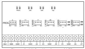
Figure 9: LX-Bus Headers and LEDs
