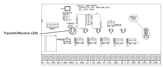
Figure 5: XR550 Series Panel Showing Reset and Transmit/Receive LEDs
