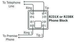
Figure 11: Phone Jack Wiring
