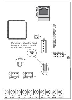
Figure 12: XR550 Series Panel Showing the RESET Jumper
