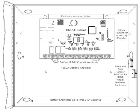
Figure 2: XR550 Series in Model 350 or 350A Enclosure
