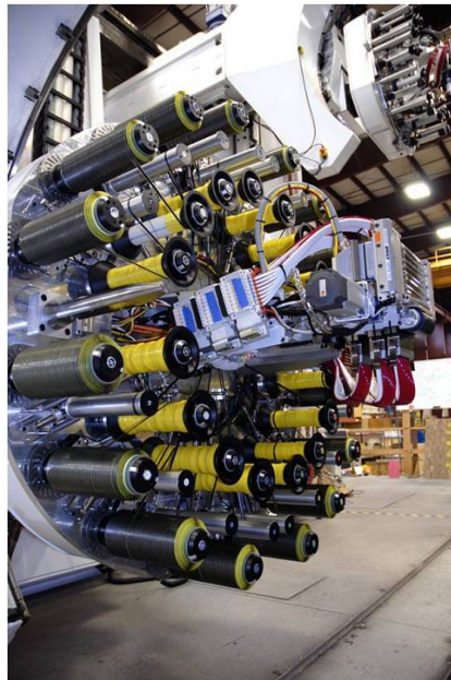
Figure 5. An Electroimpact AFP head, similar to the one now being used at Spirit Aerostructures to create the Boeing 787 fuselage section 41. (Image courtesy of Electroimpact)
