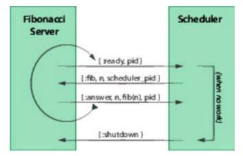
When the calculator is ready for the next number, it sends a :ready message to the scheduler. If there is still work to do, the scheduler sends it to the calculator in a :fib message; otherwise it sends the calculator a :shutdown. When a calculator receives a :fib message, it calculates the given Fibonacci number and returns it in an :answer. If it gets a :shutdown, it simply exits.
