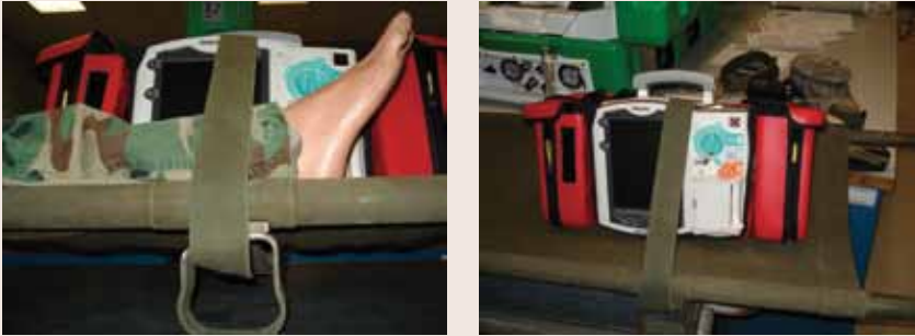
FIGURE 7. EUT NO. 2—TIE-DOWN ON A LITTER
