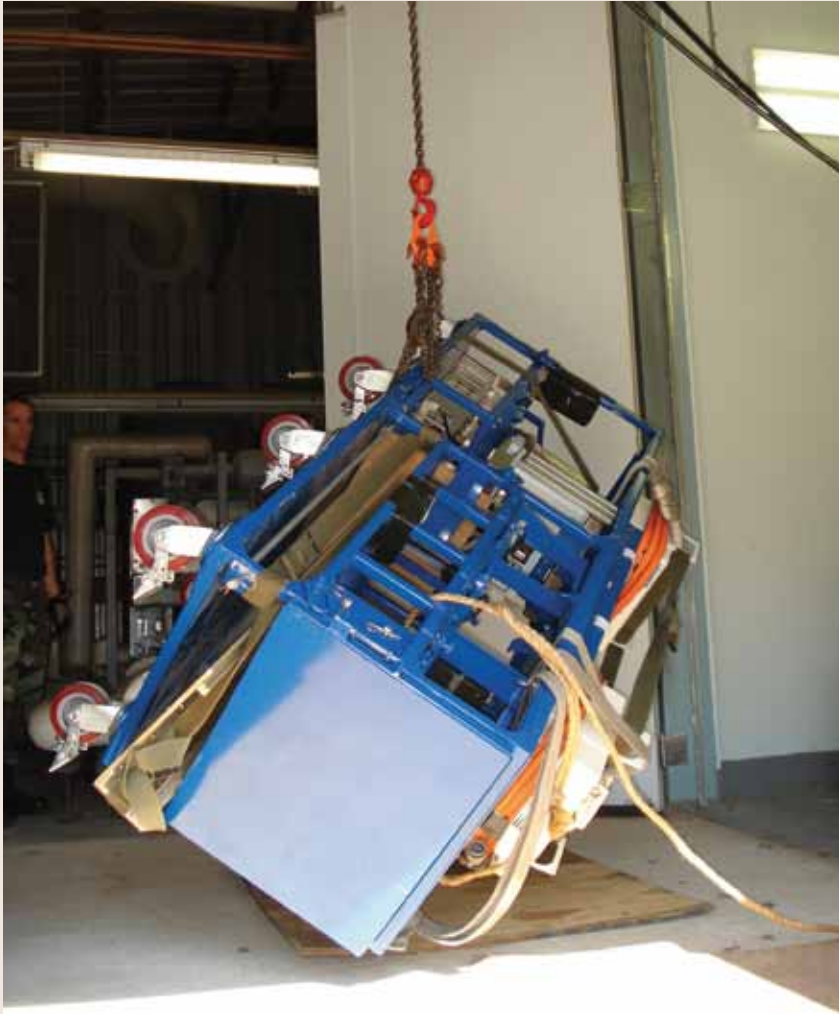
FIGURE 10. VIEW OF SUT NO. 1 DURING HANG TEST
