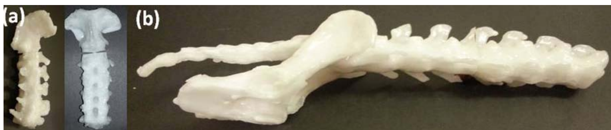
Figure 41- Printed parts: (a) cervical spine; (b) lumbar spine.
