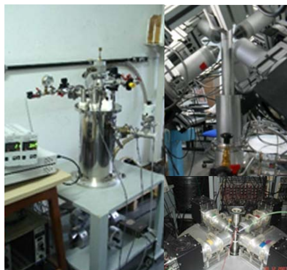
Fig 1. Closed-cycle He refrigerator at the center of a six-detector PAC spectrometer (left). He-vapor cryostat to cool samples down to 1.2 K (middle). Compact furnace at the center of a four-detector PAC spectrometer to measure samples in the range from 300 K to 1350 K (right).
