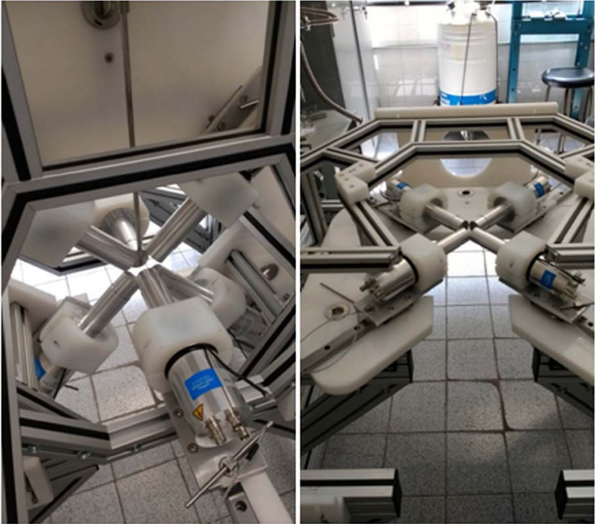
Fig 2. Reversible fully digital PAC spectrometer set up in a configuration of six \text{LaBr}_3 (left) and four \text{LaBr}_3 (right) detectors.
