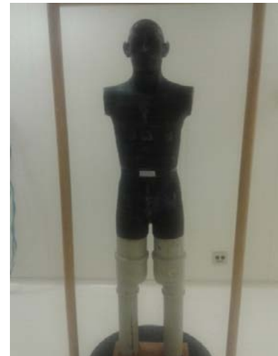
Figure 38 - Phantom AldersonRando® used in clinical electron beams dosimetry applied to Total Skin Irradiation – TSI Treatments.
