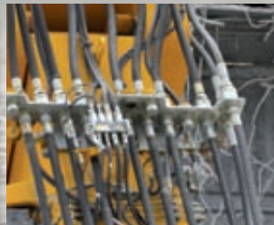
Quick release fastenings for high-pressure lines and Multifast locking system for low-pressure lines, for easy change of operating equipment
