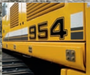
Superstructure protection prevents damage to the superstructure
