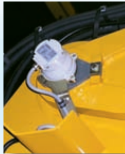
One of three LDC sensors on the attachment for permanent monitoring of the equipment position
