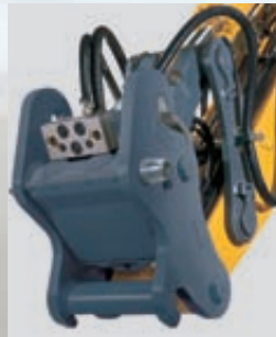
Likufix for rapid change of the add-on tools (optional)
