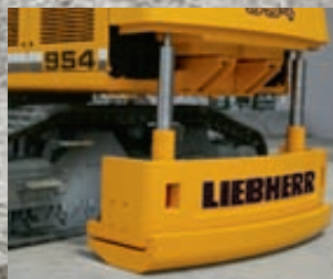
Ballast weight can be hydraulically lowered for lowering the weight during transport
