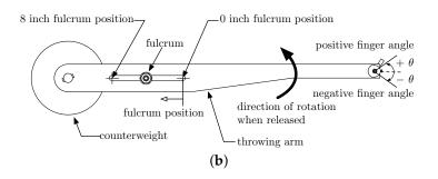
**Figure 2.** Reconfigurable trebuchet kit. (a) CAD drawing of trebuchet illustrating the four design variables; (b) measuring conventions for finger angle and pivot position.
