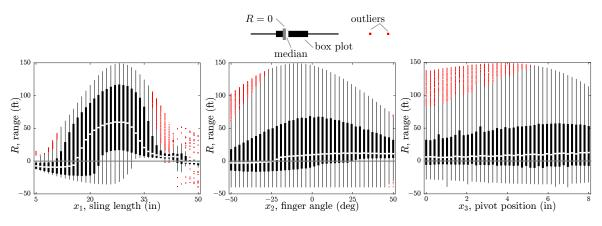
Figure 9. Sensitivity studies exploring range for each continuous design variable.
