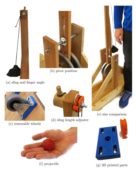
Figure 6. Photographs of trebuchet components.
