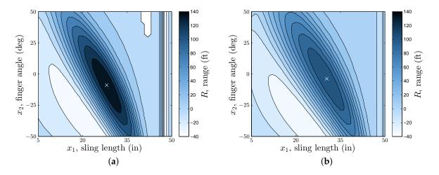
**Figure 10.** Coupling between finger angle and sling length for two fixed pivot position values. (a)  $x_3 = 4.1$  in; (b)  $x_3 = 8$  in.
