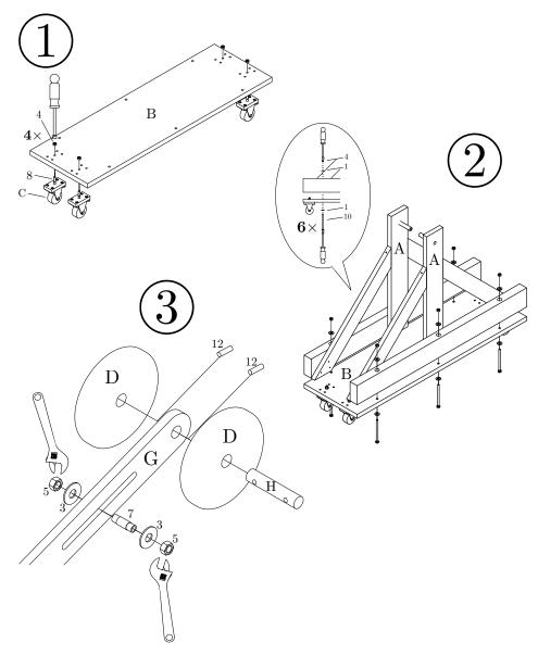
**Figure 4.** Drawings illustrating steps 1–3 in the assembly instructions. Step (1) involves fastening of casters to the trebuchet base. Step (2) illustrates attachment of upright shoulders to the base. Step (3) involves assembly of the pivot mechanism and attachment of the counterweights.
