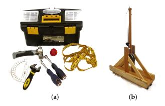
**Figure 3.** Photographs of a student toolkit and a trebuchet. (**a**) toolbox and select tools for assembly and design variable readjustments; (**b**) assembled trebuchet.
