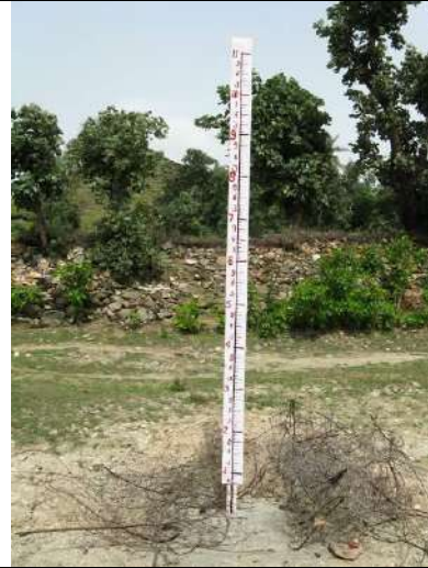
A stream gauge placed in Sunderpura village to record water level
