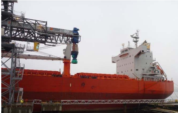
Figure 2.1-26 – Spout fully retracted (Note clearance above vessel deck)
