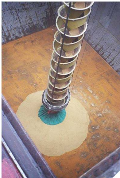
Figure 2.1-24 – Loading grain at 1 500 t/h. The shroud is lowered to allow good view of cascade effect.
