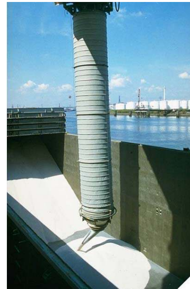
Figure 2.1-25 – Ship's hatch partially loaded with 200 tonnes of material but the floor of the hatch is clean. The spout here is provided with a rotating trimming chute.
