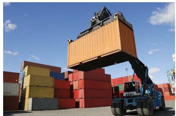
Handling of full containers with top pick.
