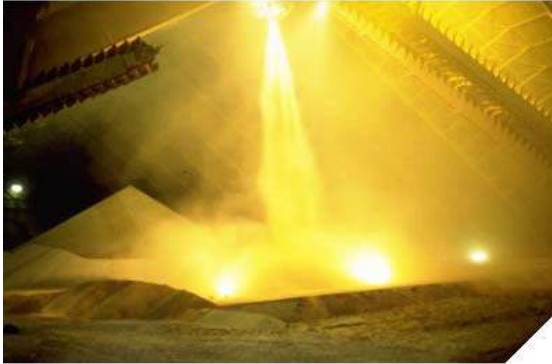
Figure 2.1-22 – Demonstration of dry bulk material in free fall where the particles of dust separate and then are lifted out and up by the air that has been pulled down by the material itself.
