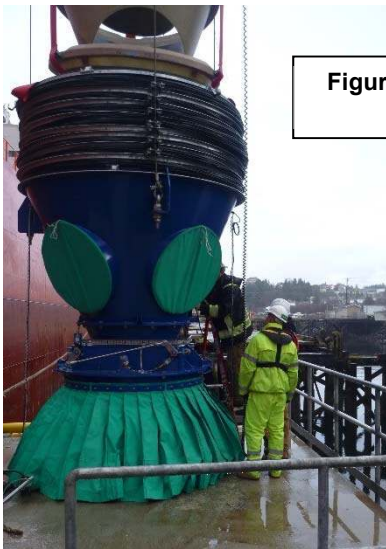
Figure 2.1-26 – Spout fully retracted (Note clearance above vessel deck)
