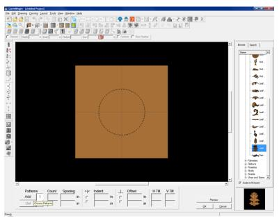
An outline of the pattern now appears along the trajectory. After the pattern has been added new options will become available. These options include Count, Spacing, Center Patterns on Trajectory, Indent, Offsets Before Projection, Offset, H Tilt, and V Tilt. Clicking and dragging the outline allows for placing the first instance in any location along the trajectory (right/left as well as above/below). The Offset and **Indent** features can also be used to alter the position of the
