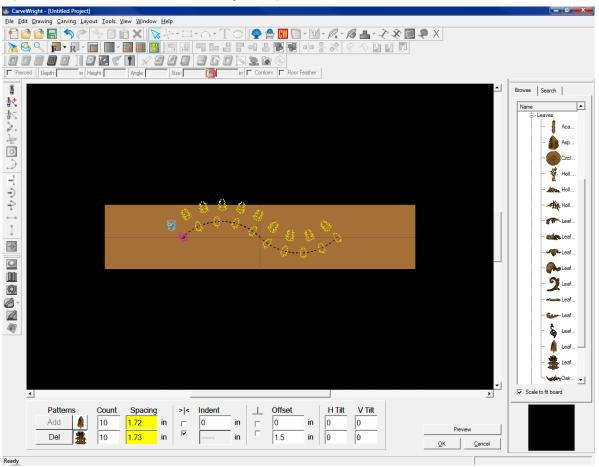
If the grouping is not centered, **Indent** allows for moving the pattern group along the trajectory. If the trajectory is open (e.g. a line or spline) the center of the first instance is placed on the starting point of the trajectory. Indenting the object will shift the pattern along the curve in the direction of the trajectory end point. Only positive numbers are allowed in the indent field.
