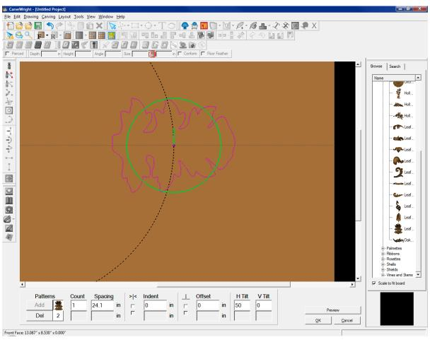
Similarly, the **V Tilt** will tilt the pattern along its vertical axis (displayed by a green arrow inside a circle showing the direction of the tilt). On a circle starting at the original three o' clock position, the **V Tilt** with tilt the left side of the pattern down into the wood.
