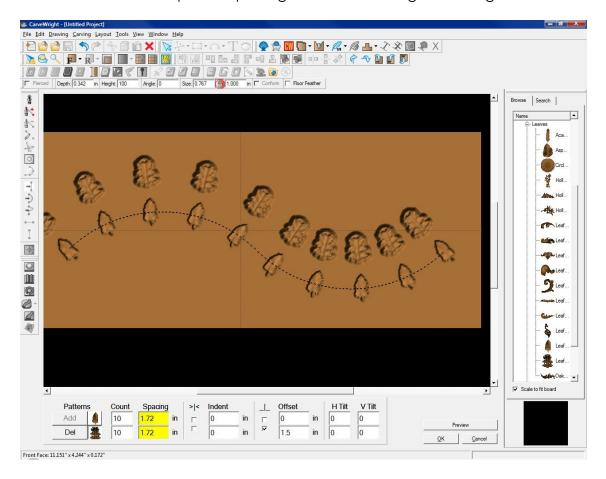
The **Depth**, **Height**, **Angle**, and **Size** tools will function the same as they would with a standard pattern addition. Once the patterns are set click the OK button and the pattern will be applied to the project and be ready to carve. To edit any part of the **Pattern Along Trajectory** parameters simply select one of the instance on the board and click the icon again.
