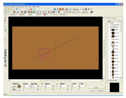
On a circle, the initial instance will be positioned at three o' clock, and as the indent is increased the pattern moves clockwise around the circle.
