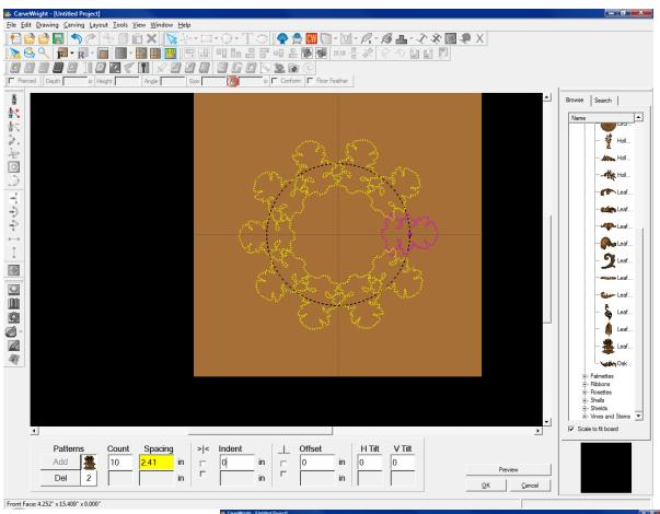
Conversely, if a number is entered into the **Spacing** input field, the number of pattern instances is adjusted based on how many can fit on the trajectory length with the given the spacing. The spacing can also be adjusted if a count is entered without altering the count as long as they can all fit on the trajectory (i.e. smaller spacing).
