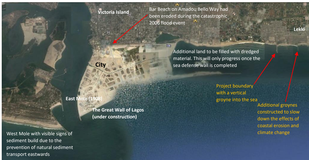
Figure 3. Overview of the current status of the Eko Atlantic project, Lagos, Nigeria
