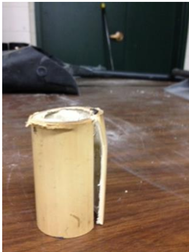
Figure 39: Bamboo Main #3 from 2013 MQP after Compression
