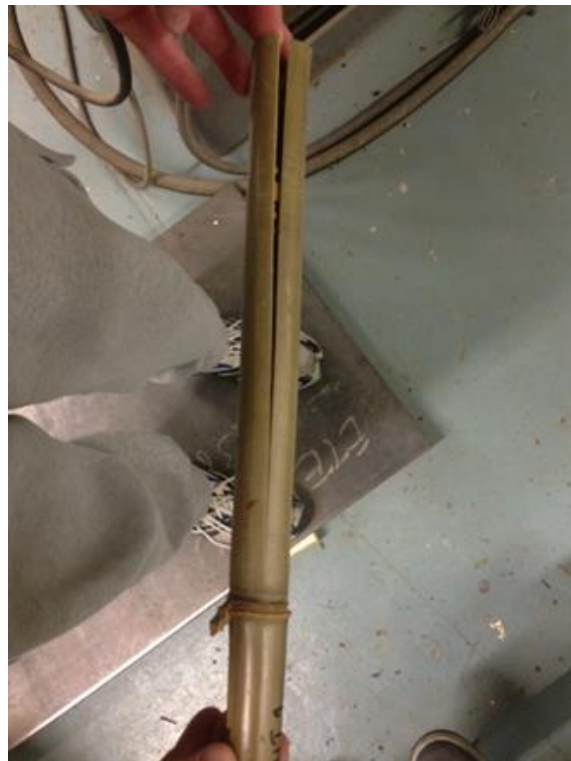
Figure 41: Heat Treated Bamboo #1 after 3 Point Loading
