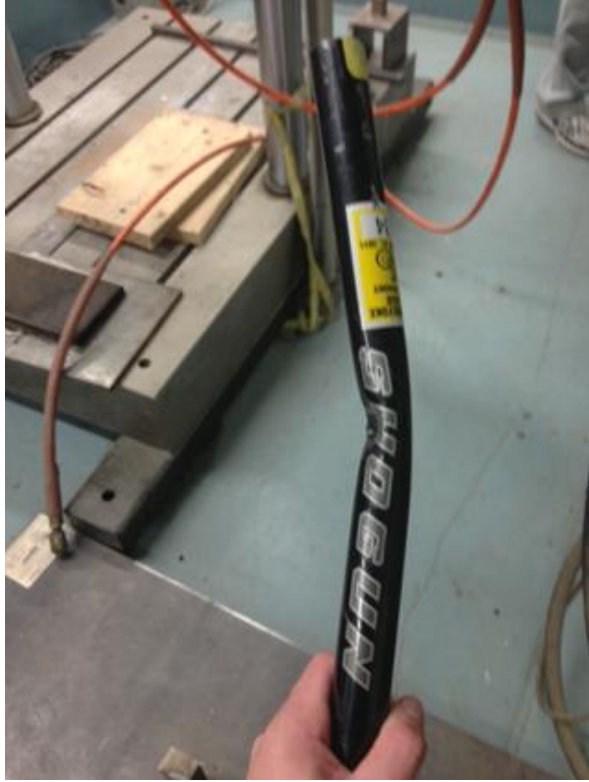
Figure 46: Steel Tubing #1 after 3 Point Loading
