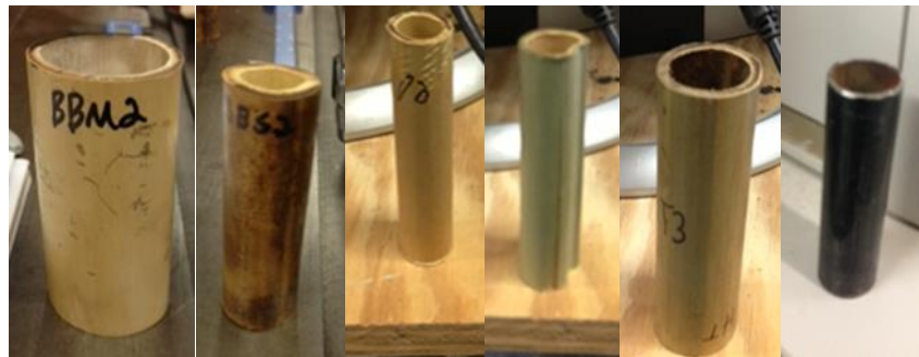
Figure 19: Bamboo from 2013 MQP Main Tube, 2013 MQP Stays, Purchased, Non-Treated, Heat Treated, and Metal Tubing (In Order)
