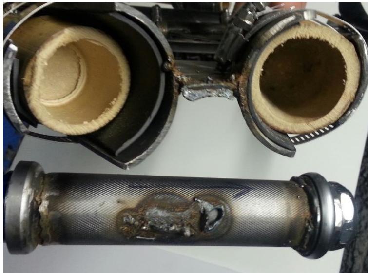
Figure 30: Failed Head Tube Weld from Frame Test
