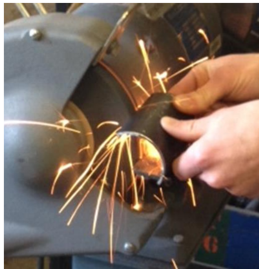
Figure 13: Bench Grinder for Final Touches
