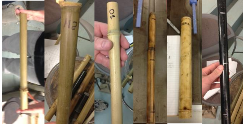
Figure 21: Heat Treated, Non-Treated, Purchased, 2013 MQP Stays, 2013 MQP Main Tube, Metal Tubing (In Order)
