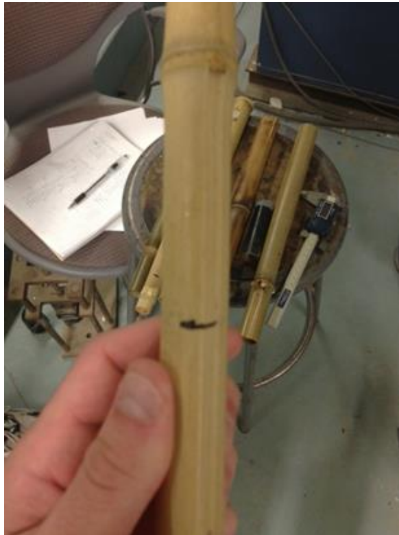
Figure 43: Purchased Bamboo #2 after 3 Point Loading
