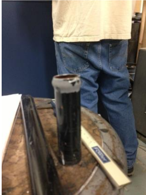
Figure 40: Steel Tubing #1 after Compression
