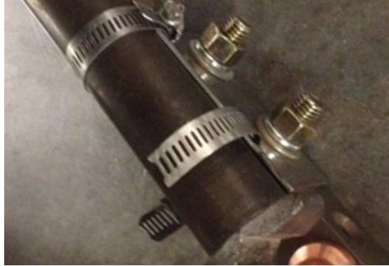
Figure 29: Failure of Hose Clamp after Testing
