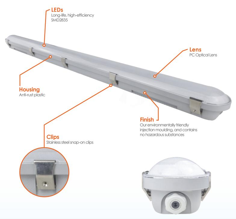
Knock-outs on both ends, connectable with waterproof connectors
