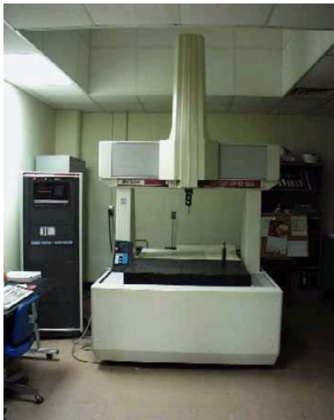
Figure D. 11: Worn die and Sheffield Cordax contact type CMM used to measure the profile of the worn die
