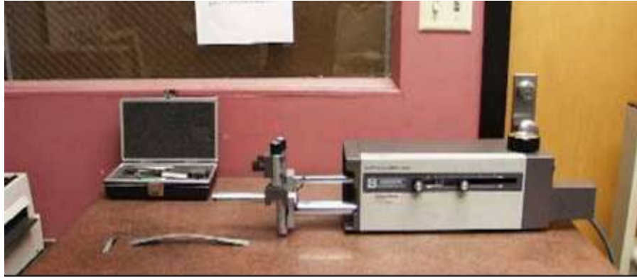
Figure A. 12: Federal Surface Analyzer used in the surface measurement
