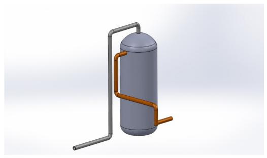
Figure 2: Proposed TES tank design
