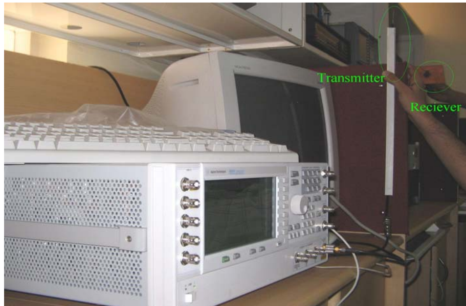
Figure – 2.17 – Arrangement for determining power received
