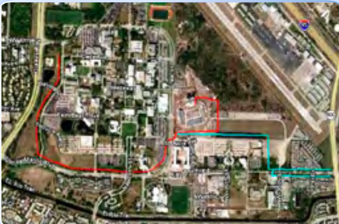
Florida Atlantic University Infrastructure Improvements Boca Raton, Florida Hypower installed 7,000 feet of concrete encased duct bank from substation to the new chiller building
