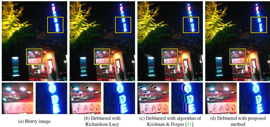
Figure 4. Deblurring saturated images. Note that the ringing around saturated regions, visible in columns (b) and (c) is removed by our method (d), without causing any loss in visual quality elsewhere.
