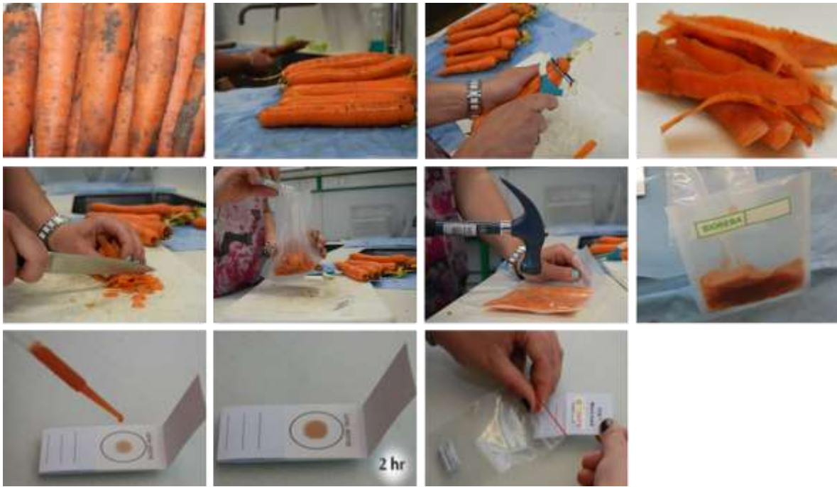
Figure 11. Sampling procedure using the NSure sampling kit. Select 25 representative carrots. Wash the carrots and collect from each carrot a vertical slice of 10 cm with a potato peeler. Combine all slices in a single compartment of the extraction bag and add the RNA extraction fluid (NSure). Close the bag and mash the pieces with a hammer to a fine consistency. Mash max. 1 min. Collect some juice from the other compartment using the pipette. Apply 2 drops of juice inside the circle on the sampling card. Air dry the card for at least 2 hours. The card must be completely dry. Insert dried card into the grip seal bag with drying agent.
