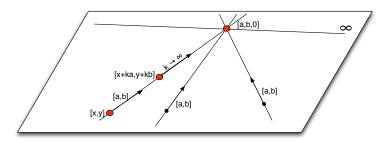
Figure 4.2: All parallel lines with direction [a,b] intersect the line at infinity at the point  $[x+ka,y+kb,1]^t \sim [x/k+a,y/k+b,1/k]^t =_{k\to\infty} [a,b,0]^t$ .
