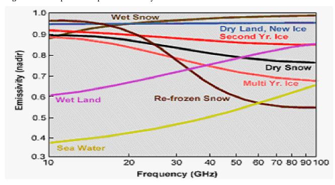
**Figure 3.3** Examples of spectral emissivity (at nadir) of some surfaces in the microwave.
