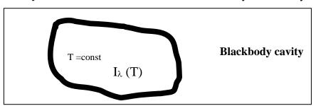
**NOTE:** A blackbody cavity is an important element in the design of radiometers. Cavities are used to provide a well-defined source for calibration of radiometers. Another use of a cavity is to measure the radiation that flows into the cavity (e.g., to measure the radiation of sun).
