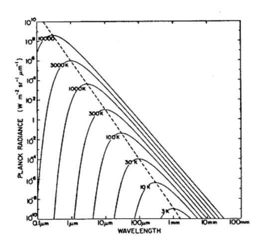
Figure 3.1 Planck function on log-log plot for several temperatures.
