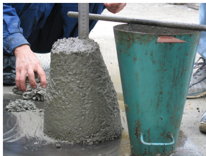
Fig. 2: Highly workable fresh concrete
