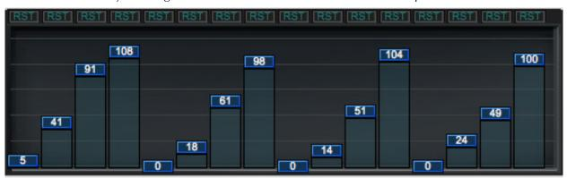
The middle section shows the 16 steps and the values of each step. While all the values may be entered in this window, there is a more convenient way to do this and will be shown below in **SEQUENCER EDITING** section.
