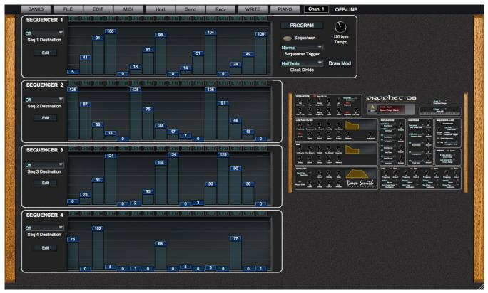
This view of the Sequencer shows the four sequencers available with the topmost set showing master functions on the right that apply to all four sets of programmable steps.
