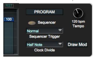
This area to the right is the master section for all four sequencers. Click on the red **LED** to turn the sequencer on and off, adjust **Tempo**, select **Sequencer Trigger** source and choose the **Clock Divide** option to determine the gate time of each step relative to the tempo.
