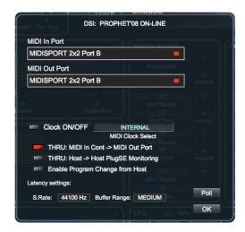
Click the **MIDI** button at the top of the Editor window. Select the MIDI interface and port that the Prophet '08 is connected to. Be sure your MIDI input and output cables are correct. Once you have selected the appropriate input and output ports, click the Poll button. An 'ON-LINE' message will appear at the top of this window confirming proper connection.
