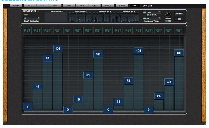
This enlarged view of the sequencer allows easier adjustment of the individual steps. The same controls appear at the top of the window along with four small windows showing the current levels of each of the four sequencers. Clicking on any of these areas will bring the values down the larger window for easy editing.
