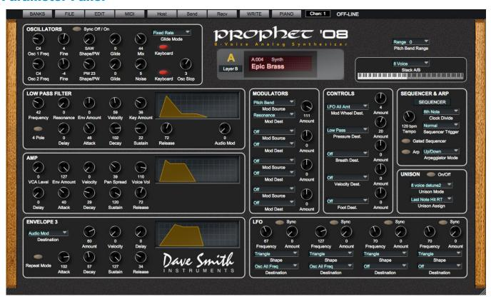
The Prophet '08 PlugSE™ Editor displays a faithful reproduction of the Prophet '08's front panel. Every knob, switch, and rotary control is exactly as you would find it on the Prophet '08, and all Editor controls are interactive and functional. Changes made anywhere on this panel will cause corresponding changes to be made on the Prophet '08 hardware, and also sent to the DAW (host) automation while recording.
