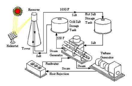
With helio-stat mirrors, solar energy is concentrated on a phase change material such as molten salt or water at the top of the tower, and stored to take care of hourly fluctuations in a thermal power plant.
