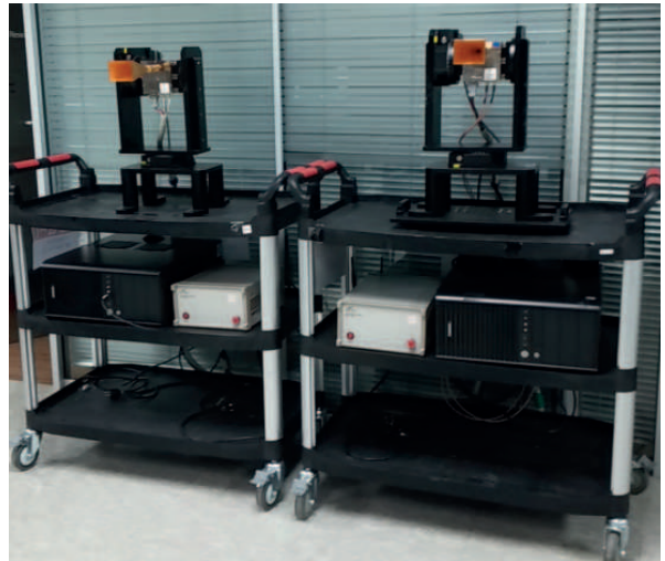
(b) Channel Sounder with Positioning Rotator
