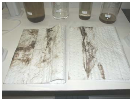
Rags used to wipe inlet and Outlet of truck pump
