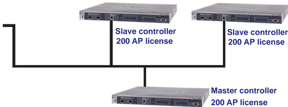
Figure 17. WC9500 stacking configuration
