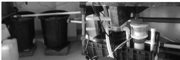
Gambar 7. Akuarium sump, a) Refungium, b) Protein Skimmer dan Fluidizer
