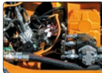
Impianto a pistoni a circuito chiuso. Closed circuit piston system.
