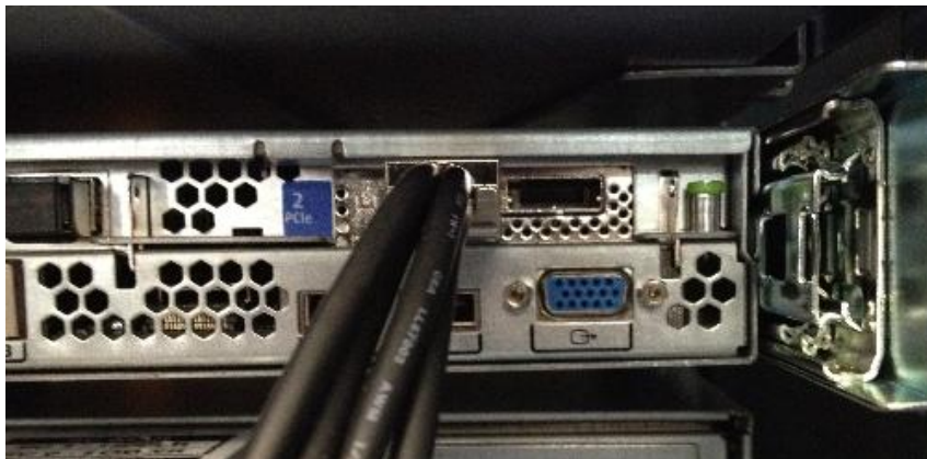
Figure 3: Rear of Oracle Server X5-2 with multi-pronged SAS cable connected to SAS HBA card.
