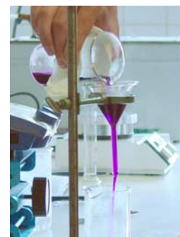
Stripping of the MnO 2 from the KClO 4 / KMnO 4 mixture
